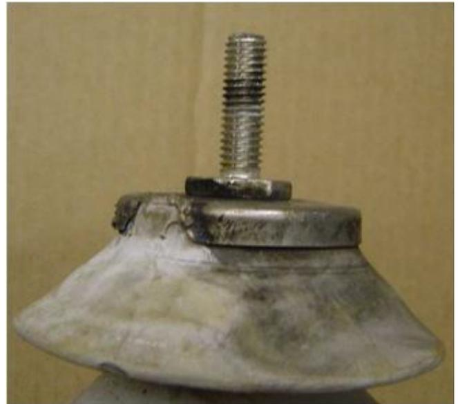
**Figure 11** Arrester where external flashover did not fail the arrester, but damaged the seal
