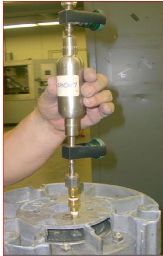
**Figure 2 Taking a gas sample of an unvented companion arrester can be very useful in the analysis**
