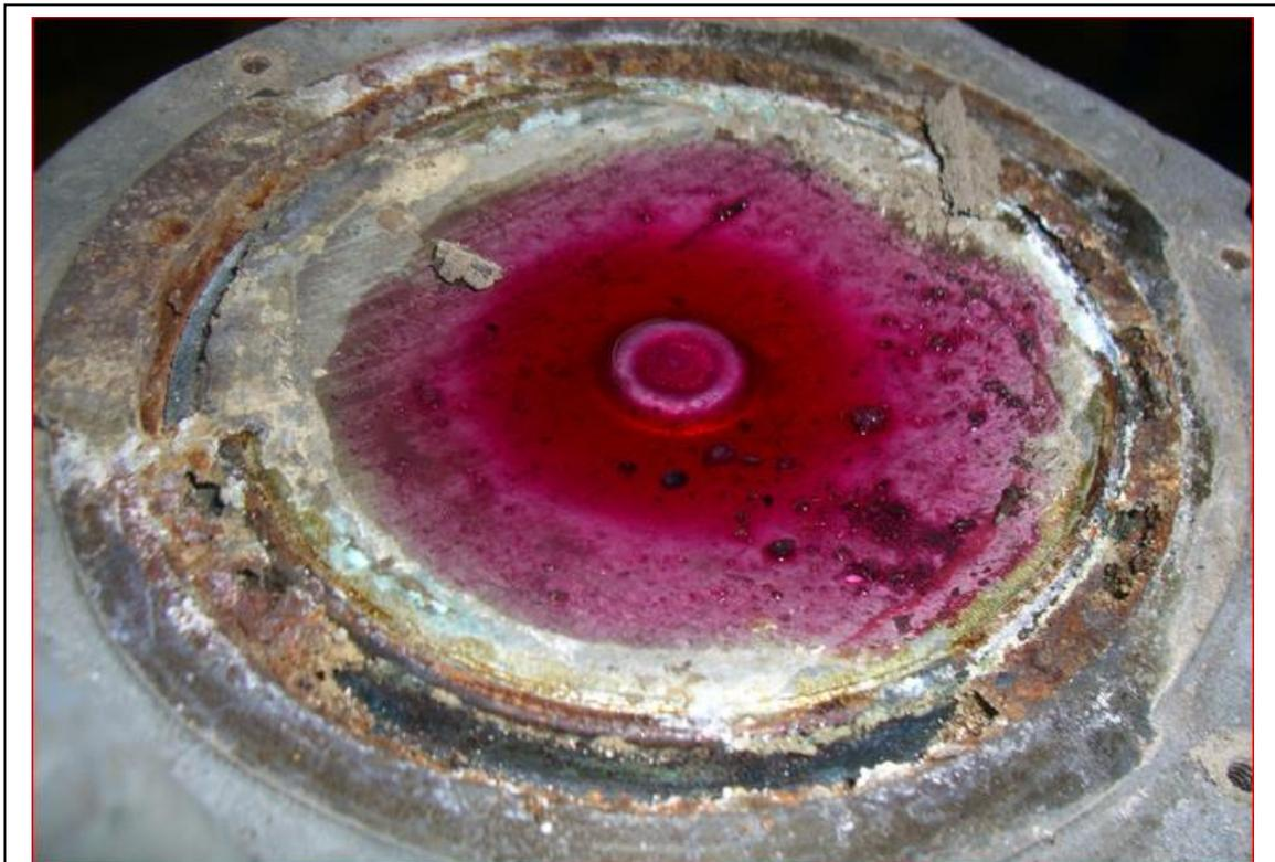
**Figure 9** Red Die penetrating fluid can be very useful in locating cracks or pinholes in metal diaphragms
