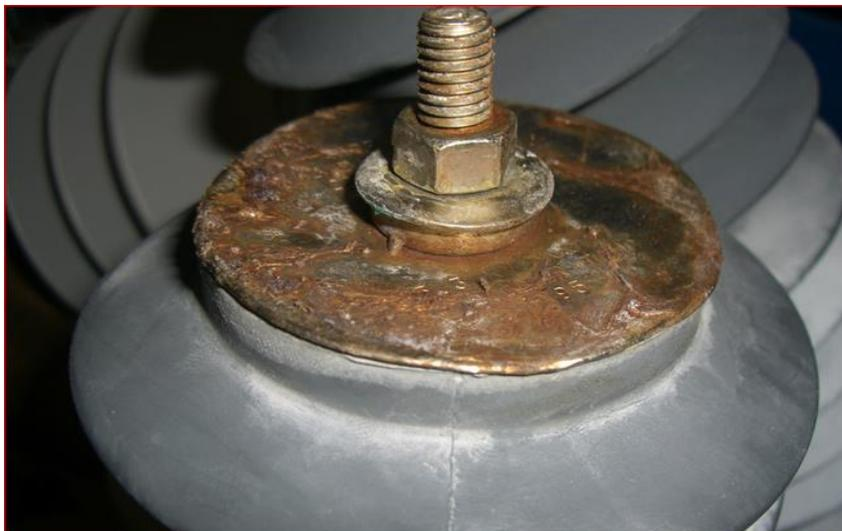
**Figure 12** Top cap with clear arc marks from an external flashover. The seal may still be good in this arrester
