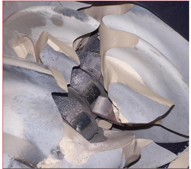
**Figure 16** Always take great caution when handling fractured porcelain, the edges are razor sharp
