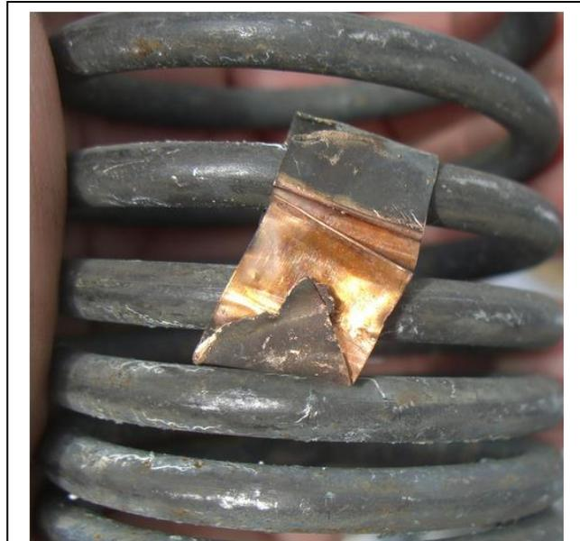
**Figure 8** Shiny copper shunt implies no moisture ingress or excess partial discharge
