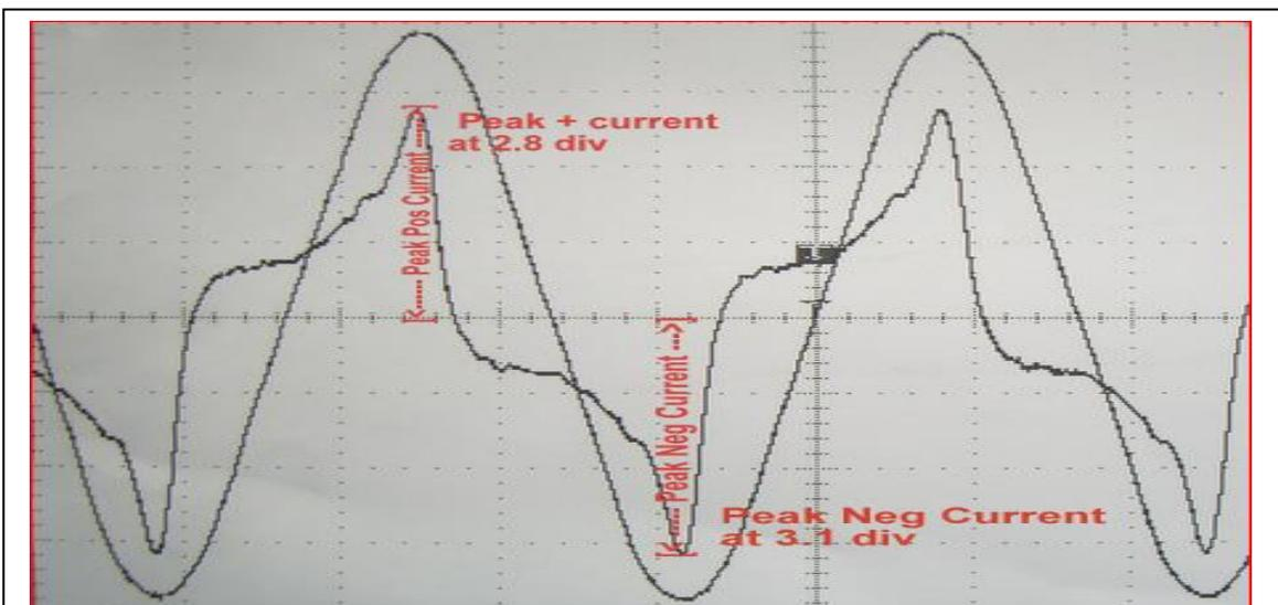
Figure 14 Example of Asymmetric Current through a surge degraded disk
