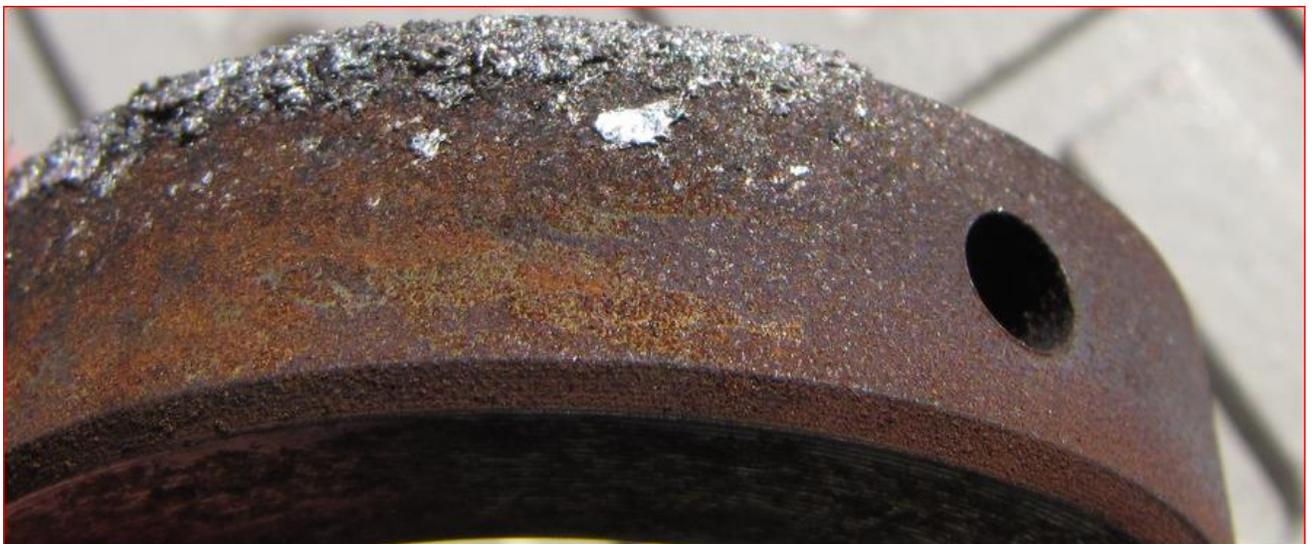
Figure 6 An internal steel component of a porcelain housed arrester that shows old and new rust along with molten metal over the old rust
