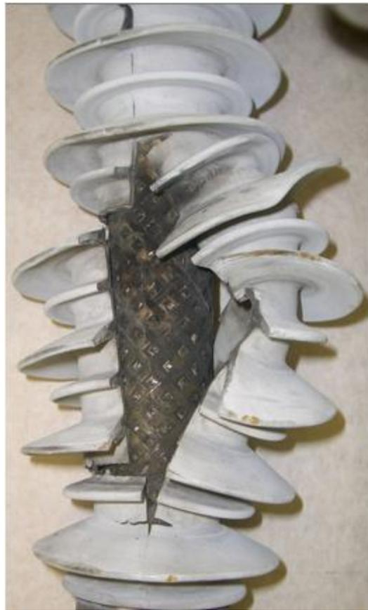
**Figure 4 Example of Non-fragmenting nature of polymer housed arresters upon overload or failure**
