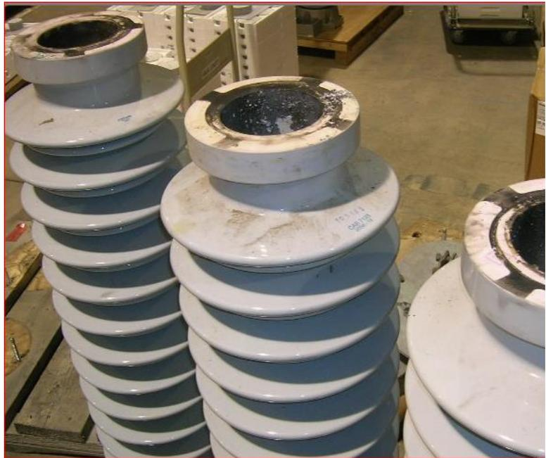
**Figure 1 Porcelain Station Arresters with internal core that has experienced a fault current event**
